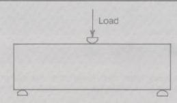
ASTM C 293 — Center-Point Loading, the entire load is applied at center span. The MR will be greater than C 78; the maximum stress is present only in the center of the span.
