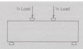
ASTM C 78 — Third-Point Loading, half the load is applied at each third of the span length. MR so measured is lower than by C 293. Maximum stress is present over the center 1/3.
