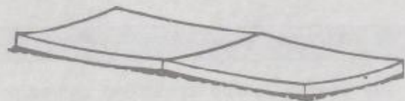
A. UPWARD CONCAVE SLABS
